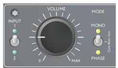
The inputs are selected by a toggle switch, the active input is displayed by a LED.
