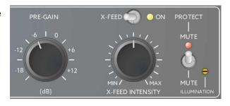
X-Feed is activated by a switch and continuously variable with reasonable amounts. The active state is displayed by a LED.
